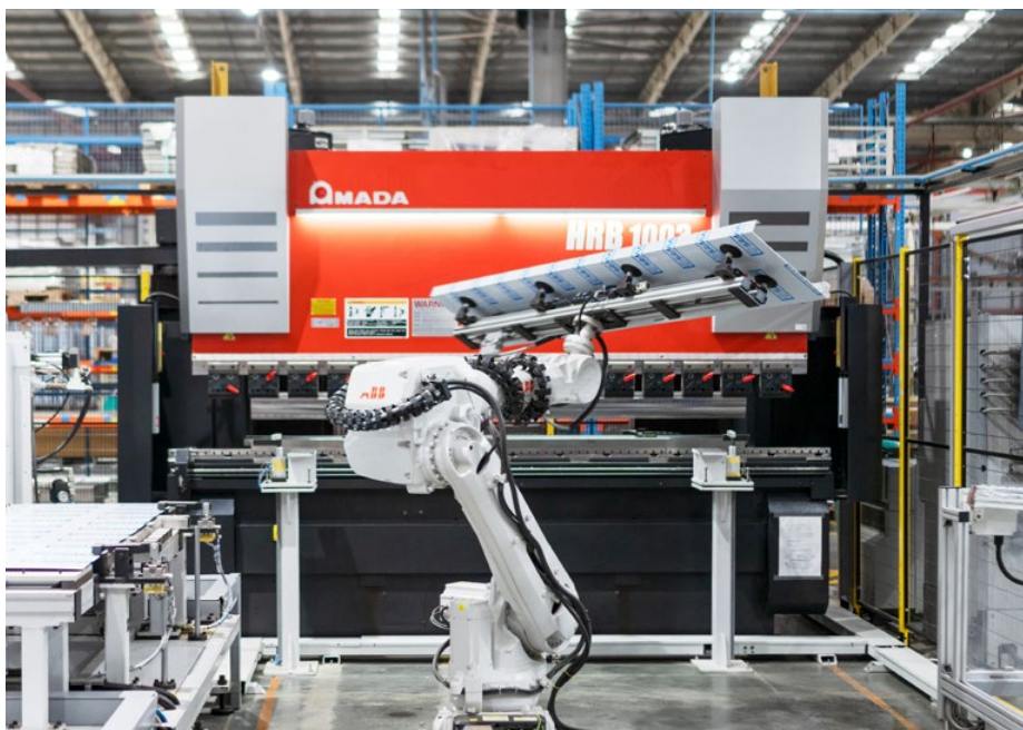
Left: High-tech support: a robot folding elevator car doors into shape.
