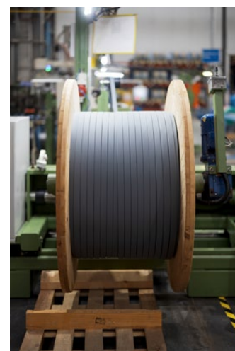
Below: Made in India for the world: belts for elevator cars.
