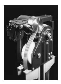
Schindler *Permanent-Magnet Drive* – the most compact elevator drive with high efficiency. It needs neither a gearbox containing oil nor a machine room, and runs with aramide or steel ropes. It is 75% smaller, only half the weight, and uses a third less energy than a traditional drive.
